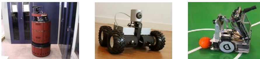
Fig. 1. B21R, WiFiBot and EyeBot robots used to develop the common communication platform.
